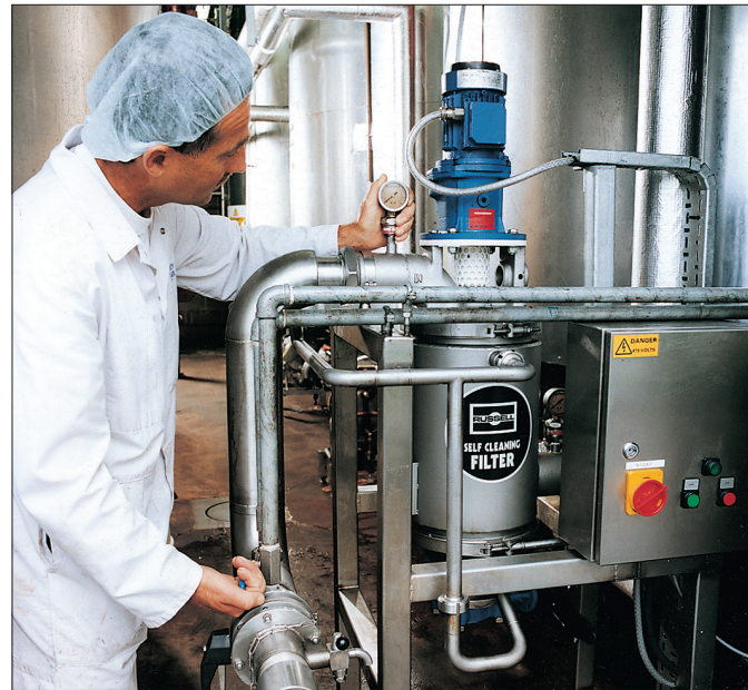
Self-Cleaning Russell Eco Filters® aid quality control procedures for filtering liquid chocolate at Walls Ice Cream.
