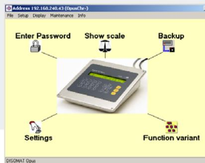
To use them, one of the 'function variants' in the instrument is activated. This puts DISOMAT into a configuration for specific applications that both allocates the essential actions to the six function keys and assigns the inputs and outputs of the instrument to the matching signals.
