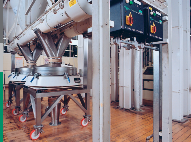
Compact 900 Sieves with Vibrasonic® debinding system at Colmans - mustard powder producer. The screens are fed from blenders and pass the sieved material through to the packaging area.
