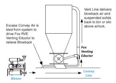
Avoiding Use of Compressed Air... Injecting Back Up the Silo/Hopper/Bin
