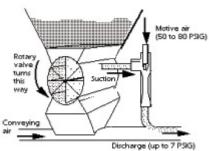
Of course, the neatest and simplest solution is for the Fox Venting Eductor to inject the blowback + suspended solids right back in the convey line. This certainly can be done.
