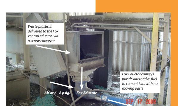
Fox eductors have been used by the cement industry since the 1980's to convey waste and alternative fuels into cement kilns. The above 8" eductor installed in the USA conveys plastic waste for combustion in a cement kiln. Other alternative fuels conveyed by Fox eductors include pet coke, dried sludge pellets, chopped tires, plastic film, sawdust, agricultural waste (rice husks, crushed oilseeds, peanut shells, ground corn cobs), shredded carpet, oil filter fluff, etc.
